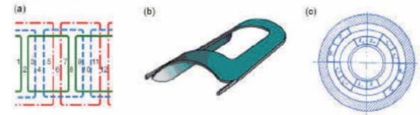
Fig. 8.34. Slotless saddle-type stator winding: (a) two-pole, three-phase winding diagram; (b) saddle-type coil shape; (3) cross section of the three-layer stator winding [10].
