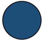
(a) Cross-sectional area available for conducting DC current in a cylindrical conductor
