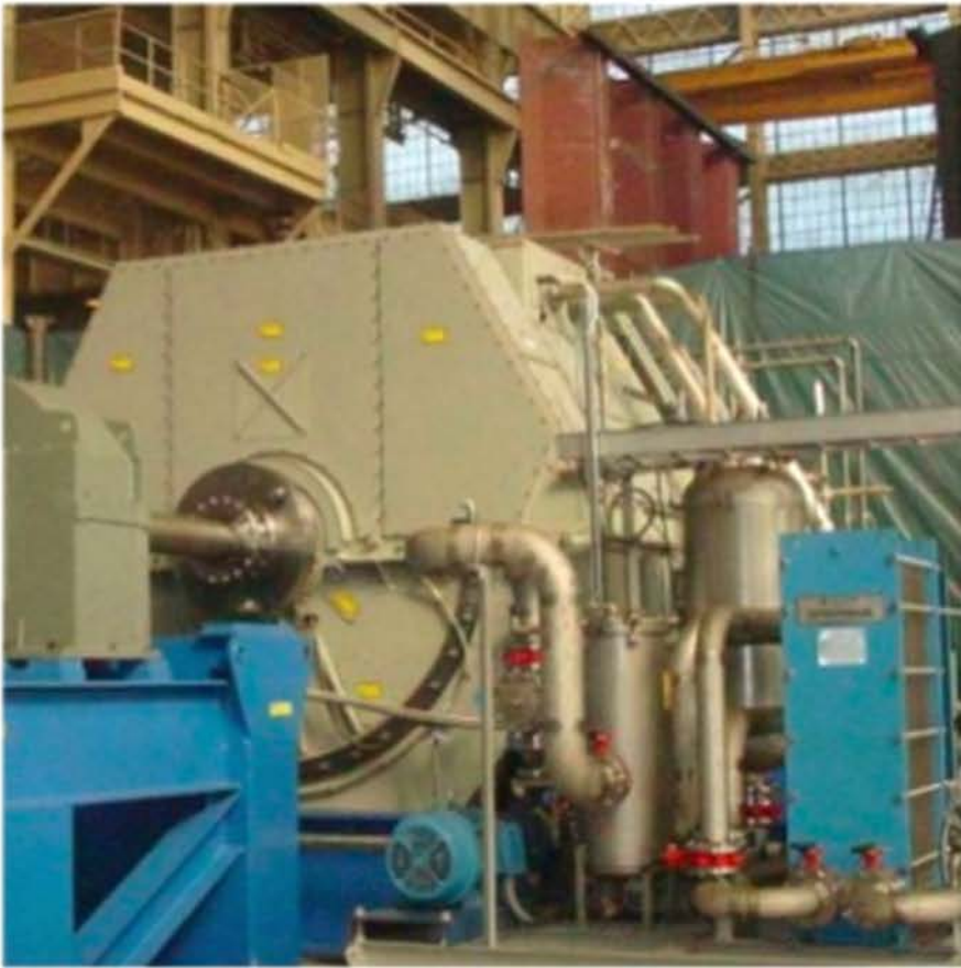
□ 36.5 MW, 120 rpm (U.S. Navy, AMSC)
