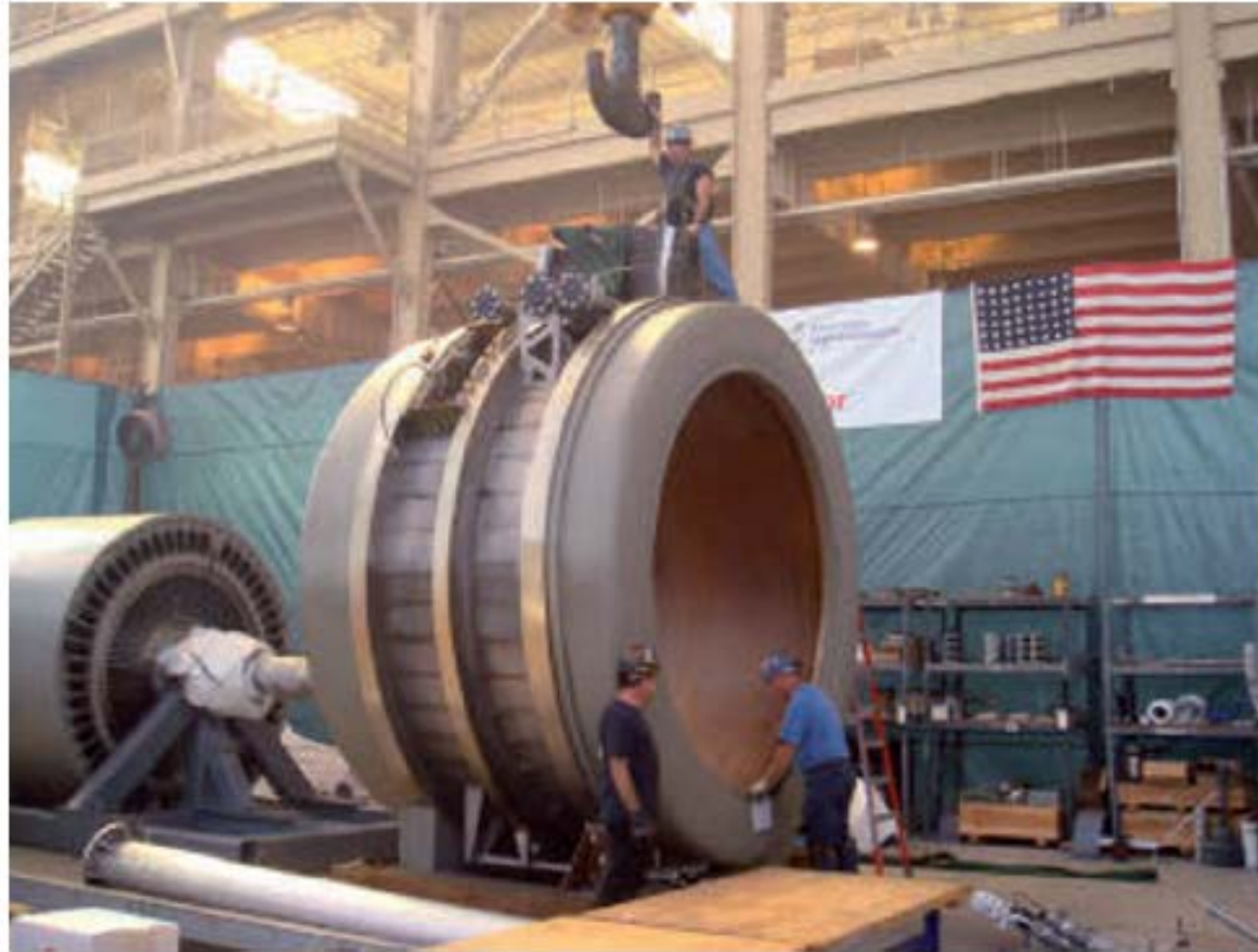
Fig. 8.13. 36.5 MW synchronous motor with 1G BSCCO HTS rotor for ship propulsion manufactured by American Superconductors . Photo courtesy of American Superconductors , Devens, MA, U.S.A.
